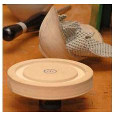
Other suggestions - leaving the stub on a roughed out bowls tenon so that the bowl could be easily recentered after it has dried out and probably turned oval, using rubber under-carpet pads for cushioning the bowl. Instead of making a jam chuck, you could use another bowl with a carpet pad between it and the bowl being returned. Turning a recess for a faceplate to sit into makes it easier to remount the faceplate again on the bowl without loosing your centering
