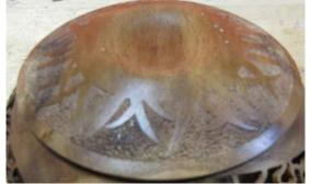
I used a flexible shaft grinder with a very small solid carbide bit. The bits are the same type as Binh Pho uses; he has them listed on his web site. The texturing is a small bit with a ball on the end. It is made by continuously tapping the wood until it is all textured
