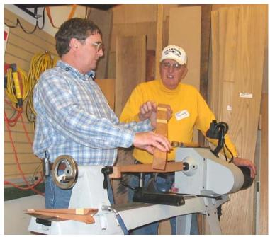
Mike demonstrated how the leg is cut and then placed off-center in the lathe for turning.
